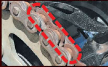
insufficient lubrication, roller wear
