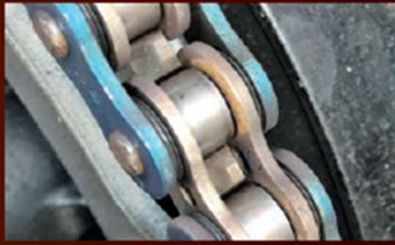
dry surface, lack of lubrication
